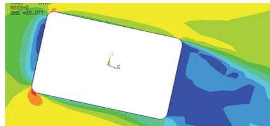
The first results of the flow analysis showed that the vacuum could cause the problem with the window failure.
